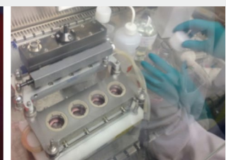
In vitro air-liquid interface device used to expose the BEAS-2B cells to the QDs ink.
